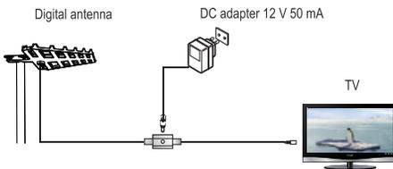
*Note: after completing the installation and installation of the antenna, adjust the antenna so that it is in the optimal position to obtain a clear image on the TV*
